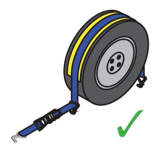
Tread style strap can be used to restrain vehicles
